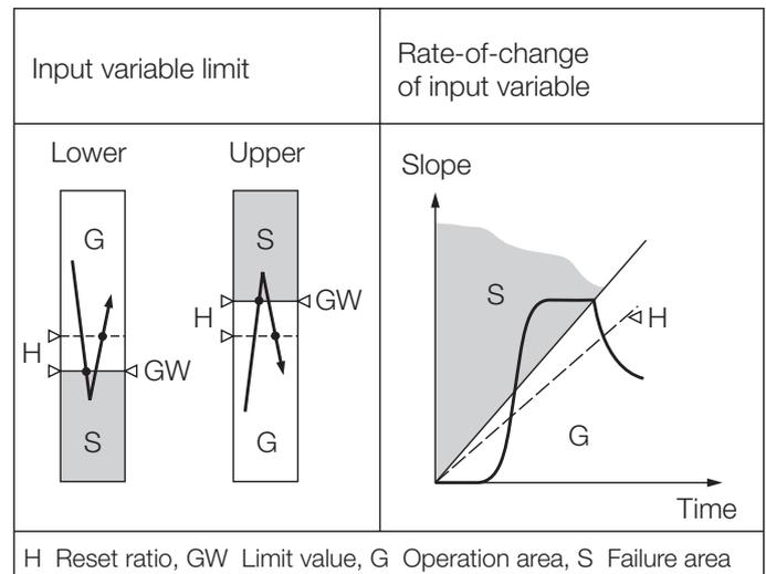
Fig. 5. Switching function according to limit monitored.
