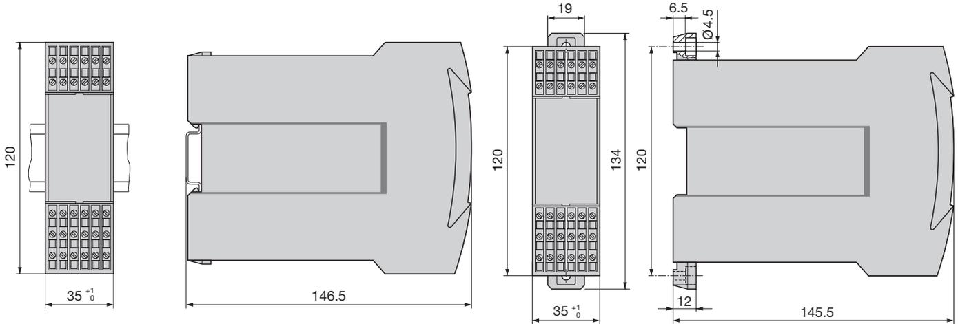
Fig. 6. SINEAX VC 603 in housing **S35** clipped onto a top-hat rail (35 x 15 mm or 35 x 7.5 mm, acc. to EN 50 022).
