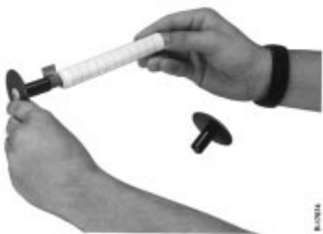
Figure 12 Removing the recording chart from the take-up reel
