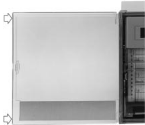
Figure 18 Replacing a door of molded material
