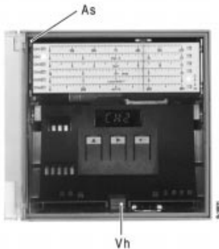
Figure 13 Removing the electronic unit
