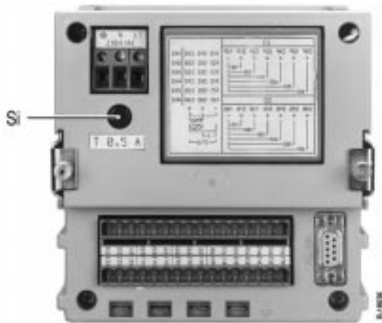
Figure 20 Replacing fuse Si
