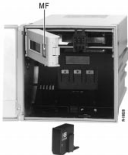
Figure 9 Placing the color head (display version)
